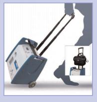
The air sampler can also be supplied in **Trolley** version: with back wheels, telescopic pole for sampling device (adjustable from 80 to 160cm) and bag accessory.
