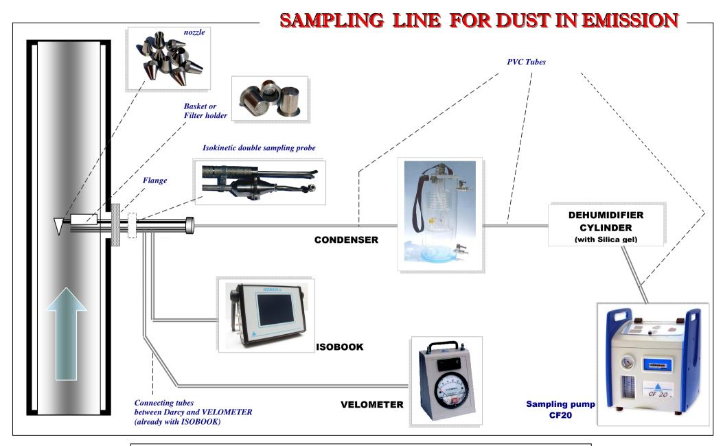
IOTE: The isokinetic probes are equipped with a filter holder but, if it is necessary, they must be completed with the basket.
