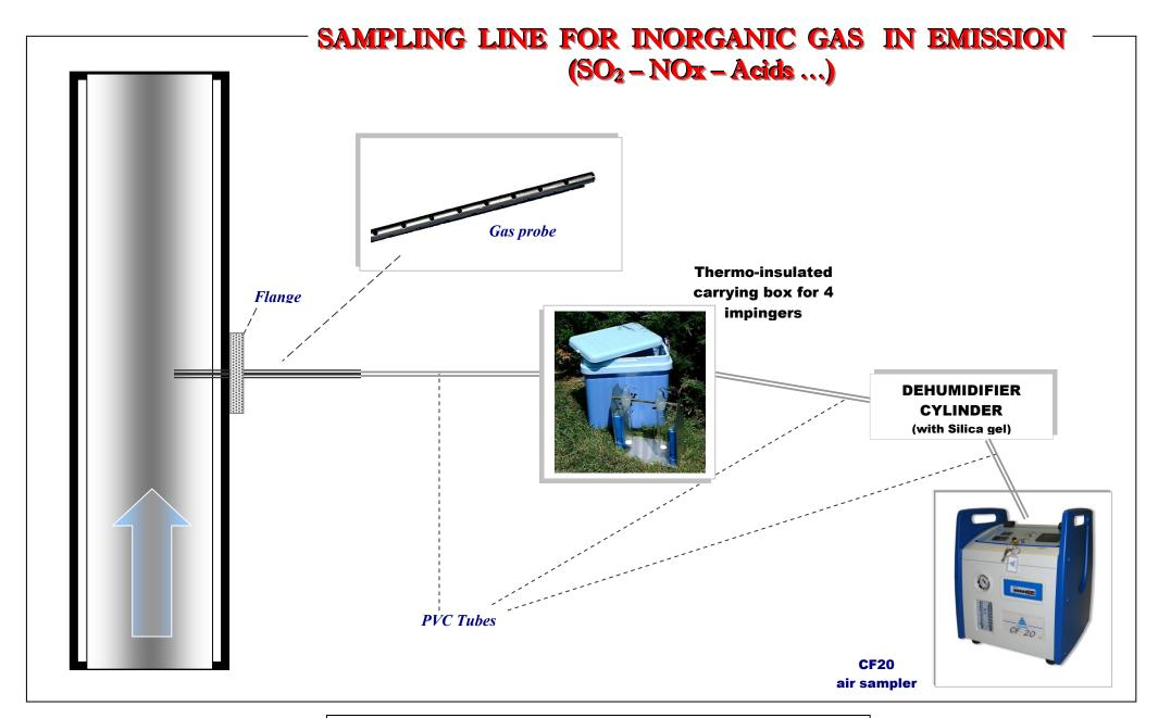
NOTE: The thermo-insulated carryng box is equipped with steel basket to accommodate up to 4 impinger
